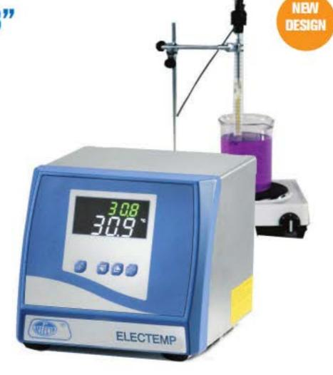
"Electemp-B" application to a hotplate, showing the unit connected with an electronic contact thermometer.
