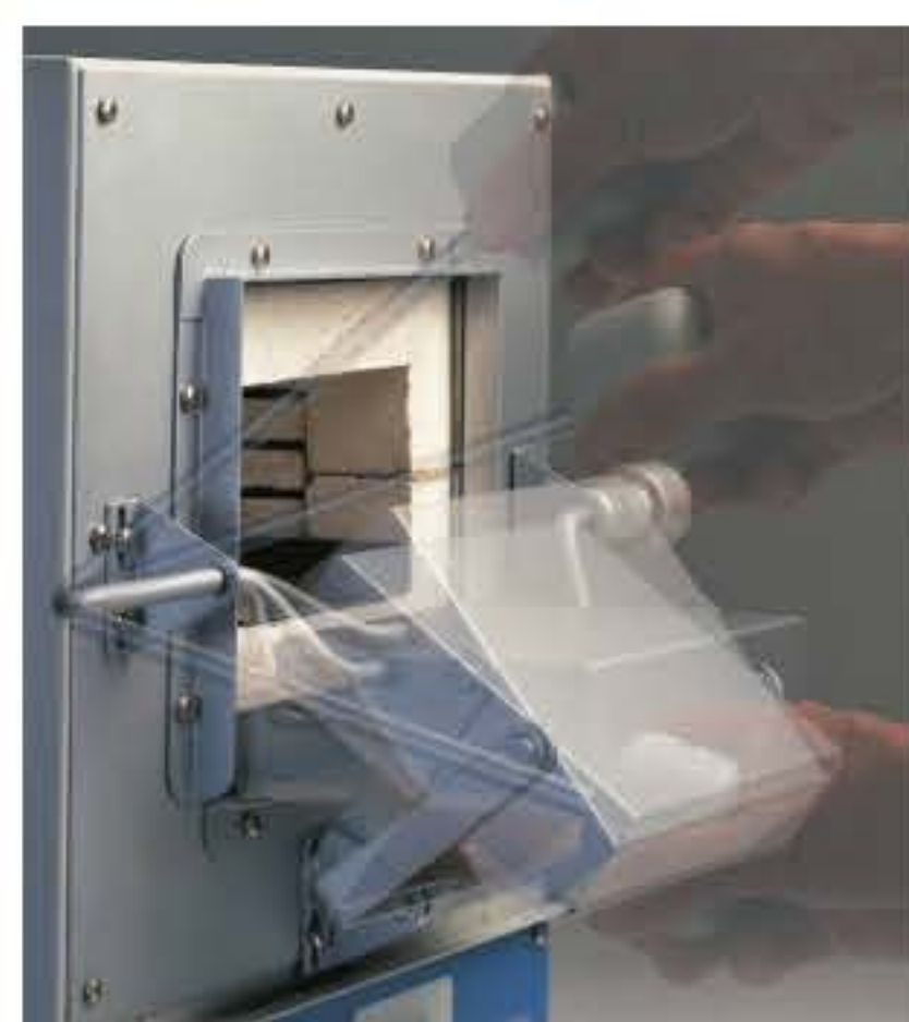
Image of the flap door system in operation.
