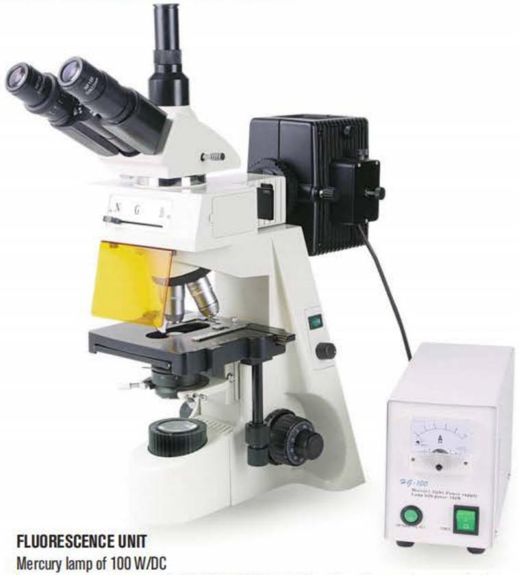
Lamp power supply connected to 110 V/220 V with intensity, voltage and power adjustable by a knob.
