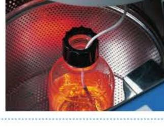
Pt 100 Sensor. 2nd Probe for reading sample temperature.
