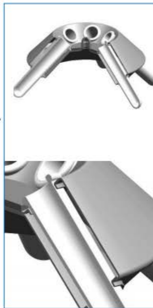
Cross section view of the angle rotor showing bucket and bucket support.
