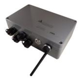
• The TRMC<sup>™</sup>-5 is a battery powered datalogger with 4G interface, especially designed for scientific field applications.
