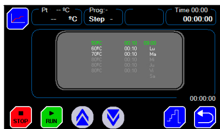
Run screen operating with temperature profile.
