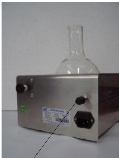
Fig. 2 Temperature probe connector location.
